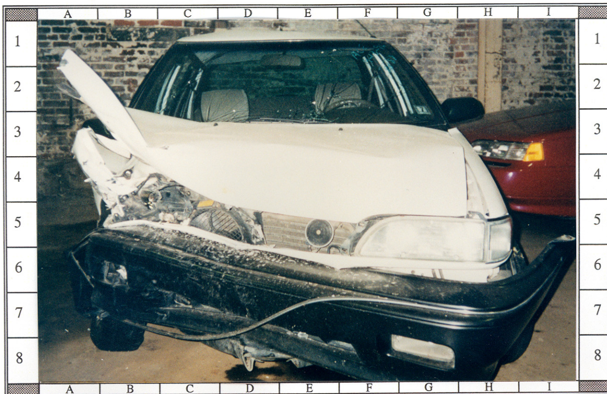
# 12: 1990 Geo Prizm's severe frontal damaged viewed from bumper line perspective; NOTE: maximum crush is at C 6 and adjustable front head restraints
